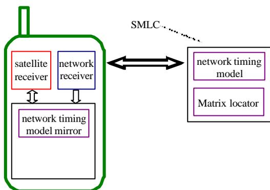
Figure 5: Elements of a network-aided Matrix-enhanced satellite terminal
