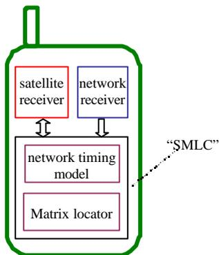
Figure 4: Elements of an autonomous Matrix-enhanced satellite terminal
